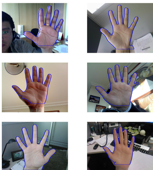
Figure 8: Examples of hand segmentation using our proposed approach.
